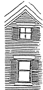
lapboarding with window detail:
